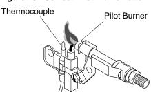
Figure 26 - Incorrect Pilot Flame Pattern
